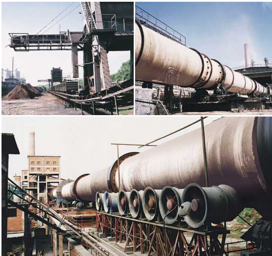
Stockpile (top left) and rotary kiln (top right) in the Nanjing cement plant. Rotary kiln in the Chongqing cement plant (bottom).
