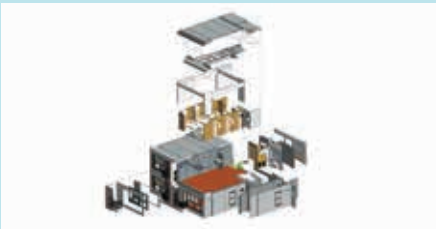
Stage 2 Designed the interior for modules prefabrication
