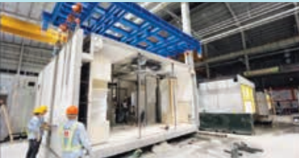
Stage 3 Factory mass production of MiC modules
